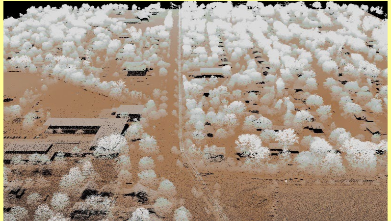
High Point Density Lidar - Please note the identification of power distribution lines.
